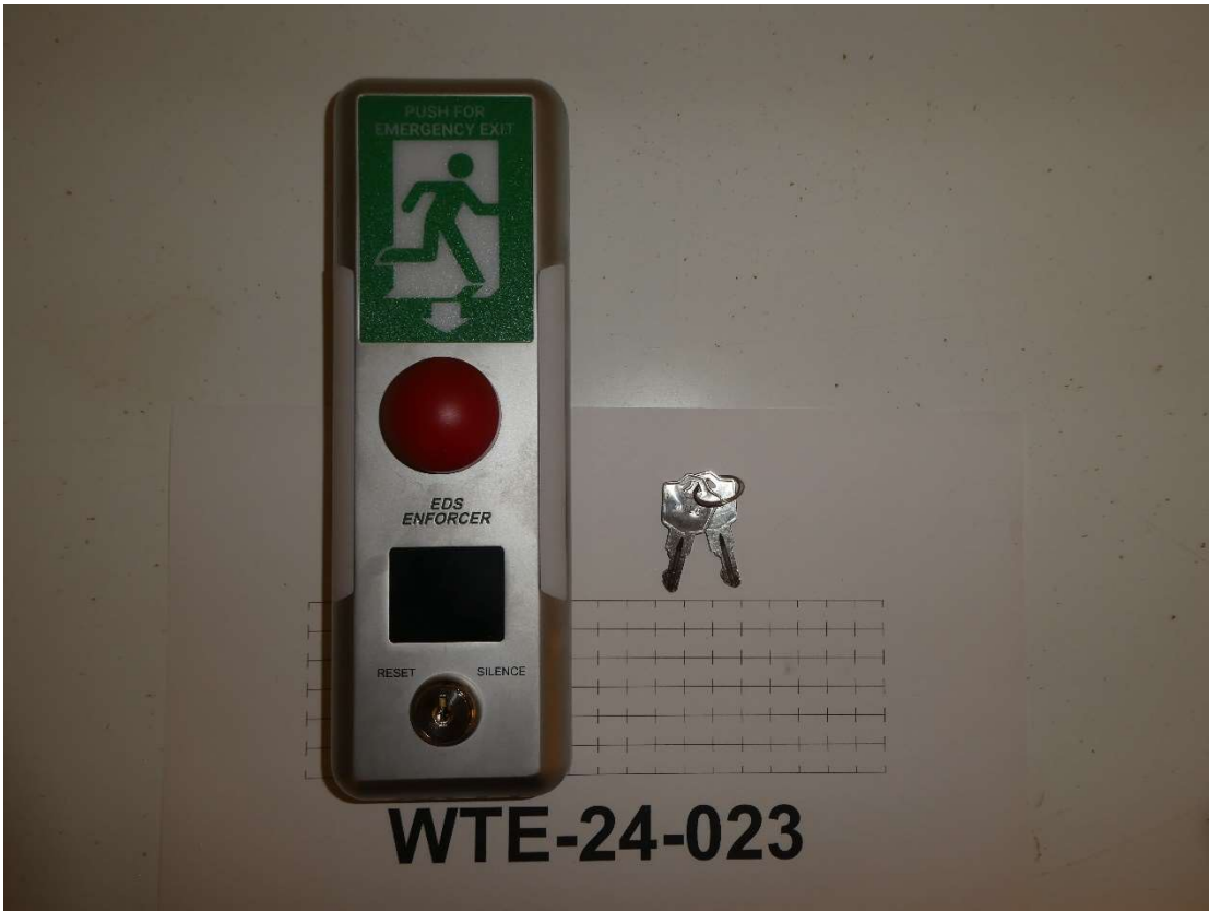
EDS Enforcer delayed egress controlling element
